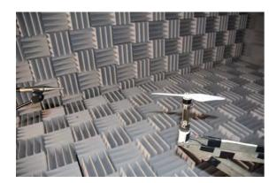
Our 22' x 17' x 7'-4" (internal dimensions) anechoic chamber testing facility is equipped with excellent acoustic attenuation with a 24 dBA ambient sound pressure level and precise Class 1 microphones. Propellers, ducted fan systems or small UAVs can be placed inside the chamber to collect data on:
