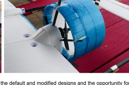
horizontal and vertical control vanes aft of the duct and moving the center of gravity aft. These changes could reduce trim drag and surface area, in addition to further take-off efficiency improvements.
