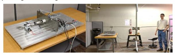
DARcorporation has completed the construction of a new Motor Characterization Stand. The newest addition to our state of the art testing lab, this unit will allow us to independently characterize a variety of electric motors for performance and efficiency. This testing capability will allow for matching of the motors to loading/mission requirements of ducted fans and propellers for integration into UAVs. Contact us for more information on our testing capabilities and facilities.
