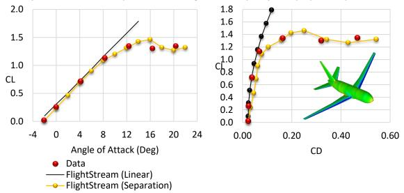
This feature also allows users to plot the locations of flow separation on the surfaces of the geometry (as shown below for the NASA XC-142 Quad-rotor VTOL aircraft), and to use this contour field variable within a trade-study tool.
