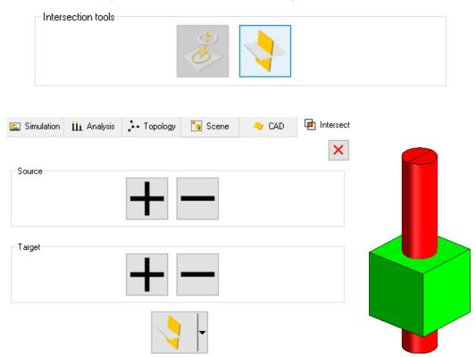
The resulting drawing curves from the intersect operation can then be used to imprint a closed loop of curves on to the target faces as shown for the sample case here. This capability can be used to repair CAD models that involve self-intersections as well as to create new complex bodies from simpler individual components.
