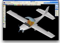
conic sections. Adjacent surfaces can be easily made exactly tangent to each other so there will be no bumps or dips in your finished airplane. This result is very important in composite airplanes with smooth surfaces that reveal the slightest errors in curve geometry, but nearly impossible to achieve with conventional or freeform curve drawing methods.
