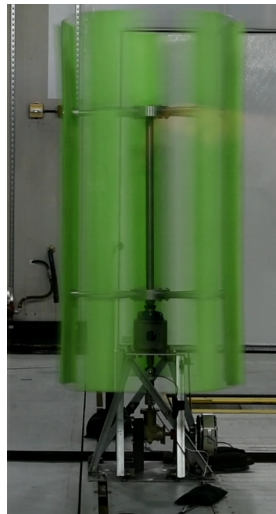
Vertical Axis Wind Turbine Test Stand
