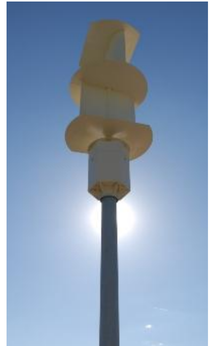
DARcorporation designed & tested Vertical Axis Wind Turbine (VAWT) Prototype for SkyDrill Power Systems.
