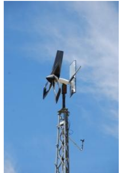
Hi-Q Wind Turbine (#61) designed & built by DARcorporation auto furled out of the wind.
