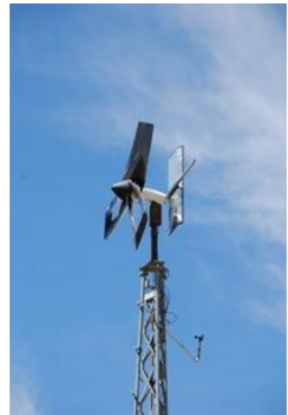
Hi-Q Wind Turbine designed & built by DARcorporation auto furled out of the wind.
